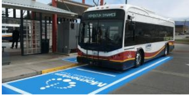
Momentum Dynamics Inductive Charging. Source: electricdrive.com
