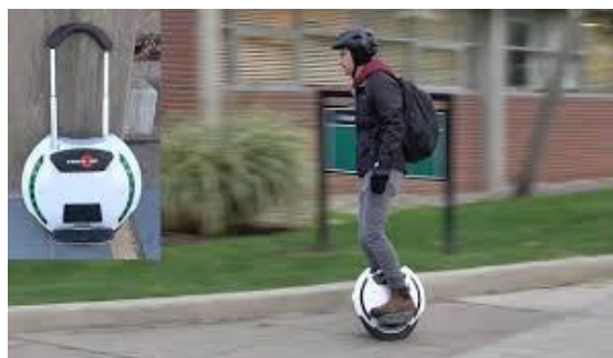
Electric unicycles can achieve 20 miles per hour and travel up to 30 miles on a charge.
