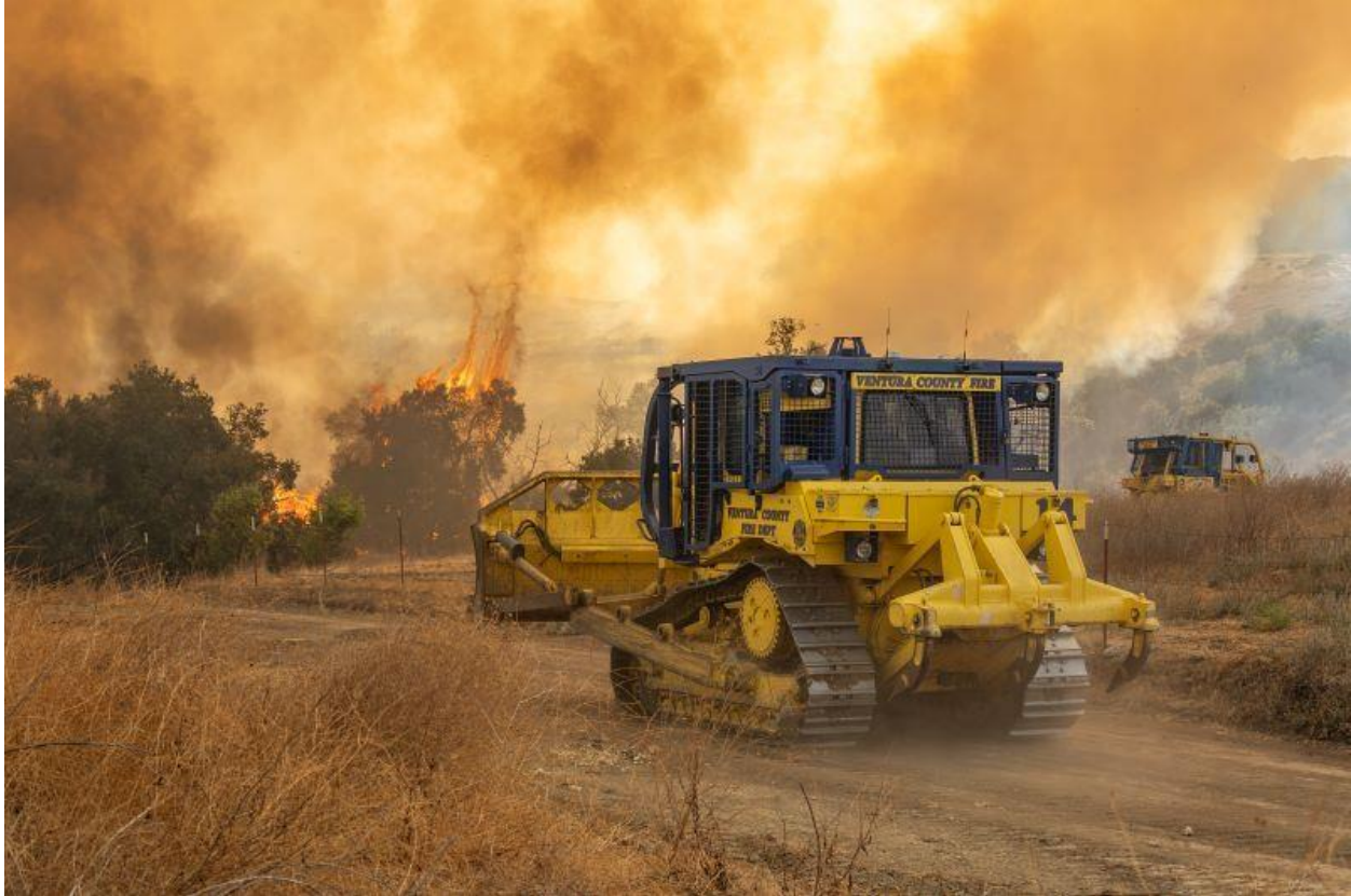
Figure 3. The Ventura County Fire Department used bulldozers to cut containment lines after the Balcom Canyon fire. (Photo courtesy of VCFD)
